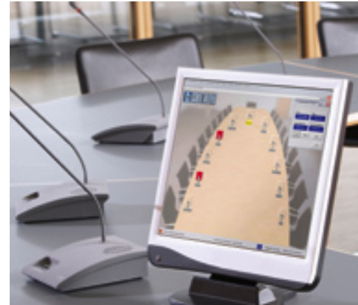
MCW-D controller software on a PC touchpanel
