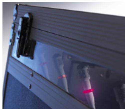
Battery status is indicated via the illuminated rings of the microphone unit
